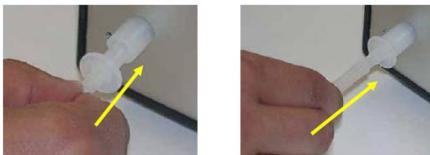
Fig. 10: Connect tubing here to vent any vapors exiting the degassing chambers to waste
